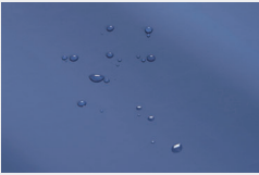
Top Cover Provide low shear, low friction, vapour permeable, and moisture protection with a basic level of flame retardancy.
